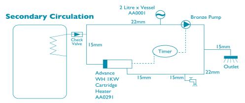
Set the WHI at 45°C to maintain temperature in the secondary loop without affecting the store temperature, costing just pennies per day.
