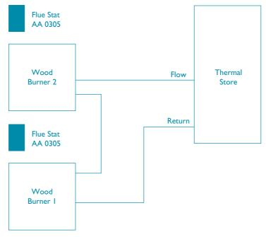
The flue stats are wired in parallel and can be pre-wired on request
