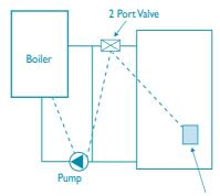
Wired in series so cylinder thermostat on demand will activate the boiler and OPEN the motorised valve (normally closed version)
