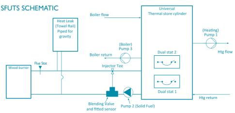
This schematic is for solid fuel pumped circulation.
