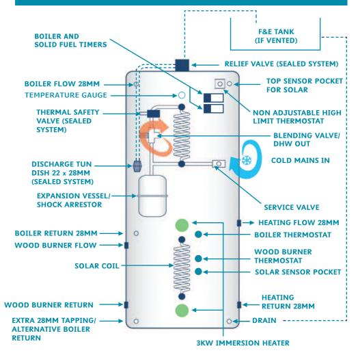
IMPORTANT: Gravity circultation must be achievable through the store from the woodburner. The store must be on the same level or higher - see diagram on page 6.
