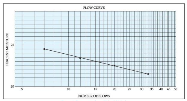
Figure 2 Determination of Liquid Limit
