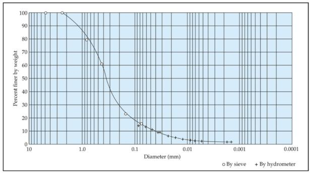
**Figure 1 Typical Grain Size Distribution Diagram**
