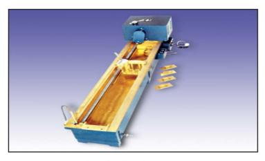
**Ductility Test Apparatus**
