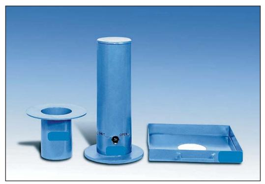
SAND POURING CYLINDER APPARATUS
