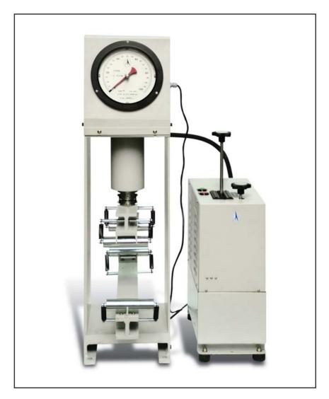
FLEXURE TEST APPARATUS
