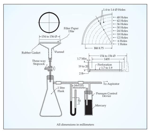
**Figure 8 Apparatus Assembly for Water Retention Test**
