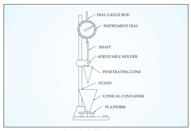
**Figure 7 Standard Cone Apparatus**
