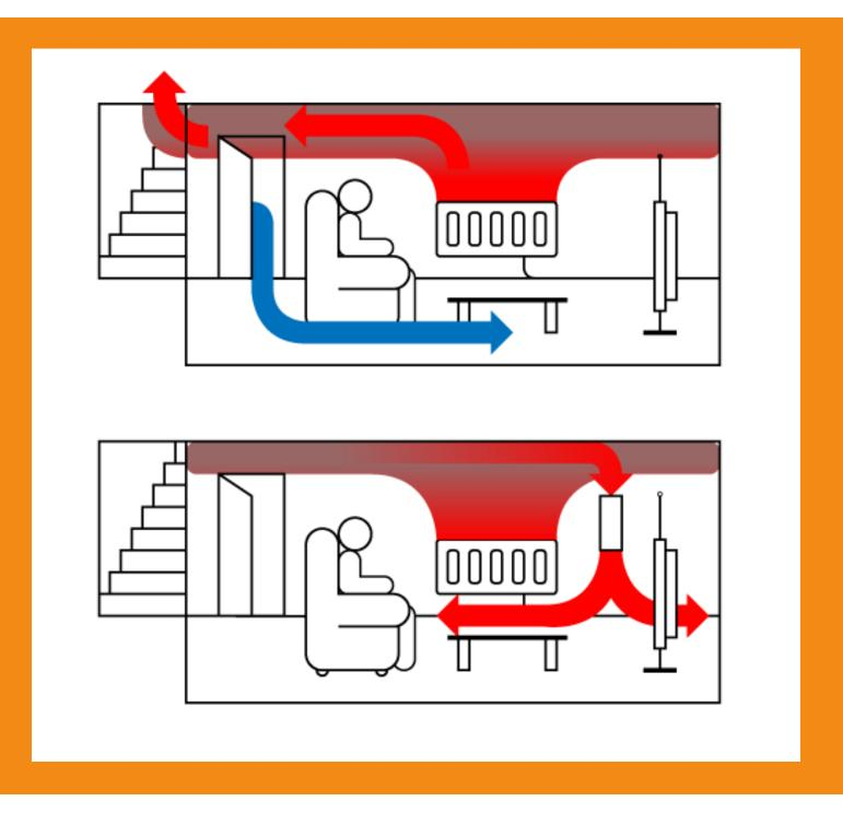
Using proven principles of destratification used widely in large buildings, airports and sports halls Tibio recirculates over 720\* cubic metres of pre-heated air daily from the top of the heat gradient at ceiling level.
