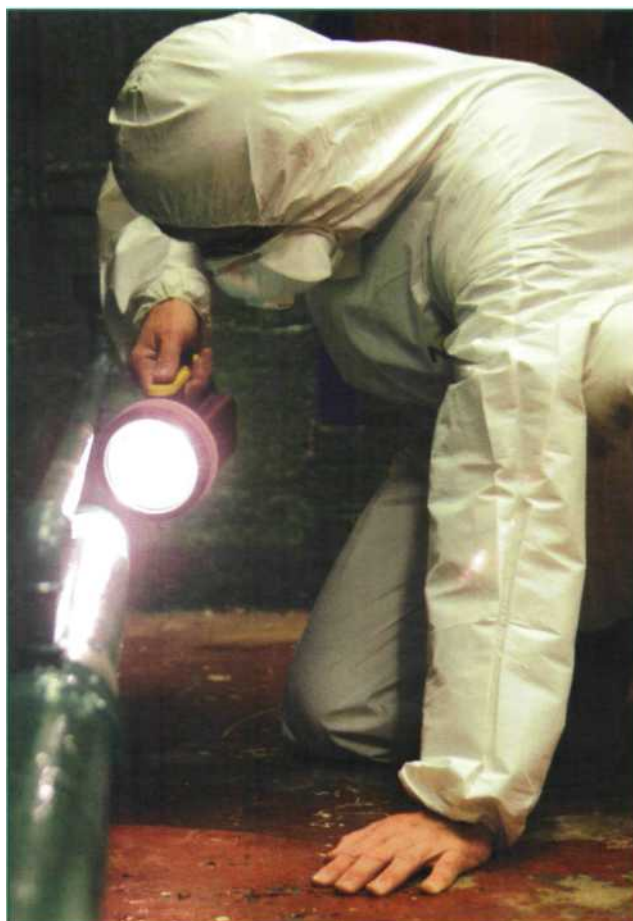
Figure 6.2 Analyst carrying out a visual inspection inside an enclosure
