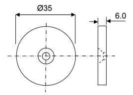
Fix with M5 countersink screw, (not supplied).
