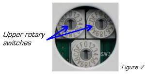
Select the required site code by rotating the switches until the arrow on the actuator points to the correct number.
