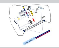
SR710S relates to the substrates they are able to measure. The IG710S captures diffuse-reflected energy, while the SR710S makes use of the reflectivity of metallic substrates to direct infrared energy through the coating.
