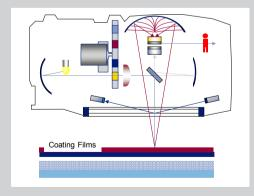
the beam to the secondary detector, to form the reference signal against which the light will be compared.
