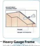
High security 2 part frame system allows for highest security, the first part is fitted in situ and the second welded to it on site to protect the fixing points.
