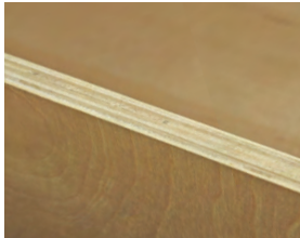
5/8" thick furniture grade veneered plywood end panels
