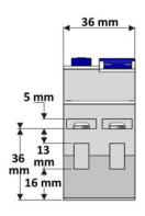
The Rtec range provides combined residual current (earth leak) protection and overload/short circuit protection in a single device and can be used to replace an RCCB/MCB combination.
