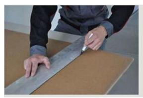
Measure and mark cutting line Process on stable war< surface - adhere to occupational safety'
