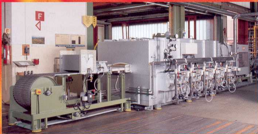
Type 11 BdG 60/34 GP furnace with gas quenching for hardening drills; gas-heated.
