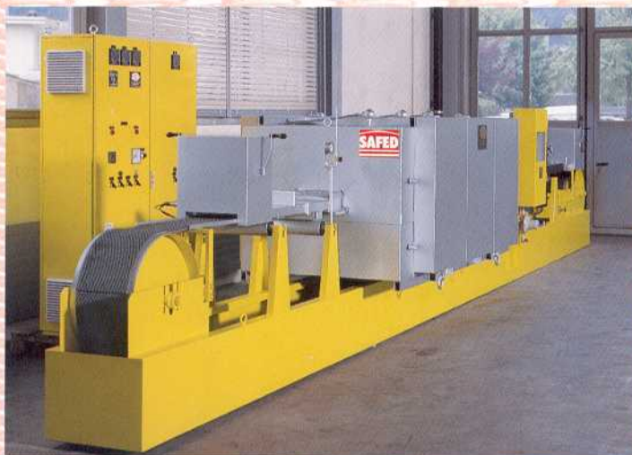
Furnace type 11 Bd 30/21 for hardening knife blades; electrically heated.
