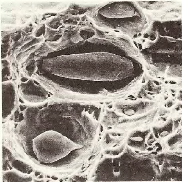
Figure 8.6 (a) Section through growing fibrous crack showing formation of notes around inclusions, but not around pearlite ( \times 240 ). (b) Fracture surface, showing void formation around inclusions ( \times 800 ) (both courtesy of R. F. Smith)
