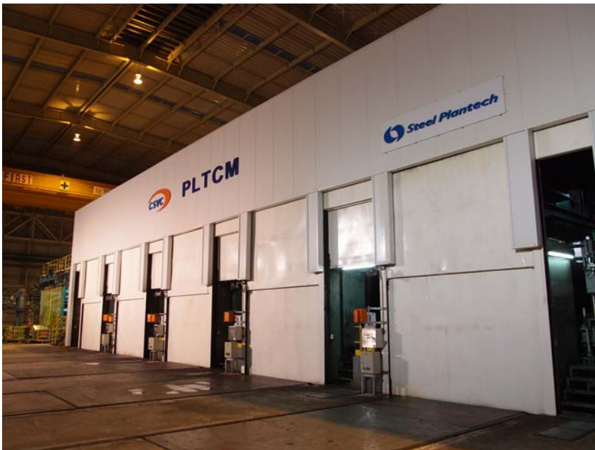
Figure 3 Five (5) stand Tandem Cold Mill
