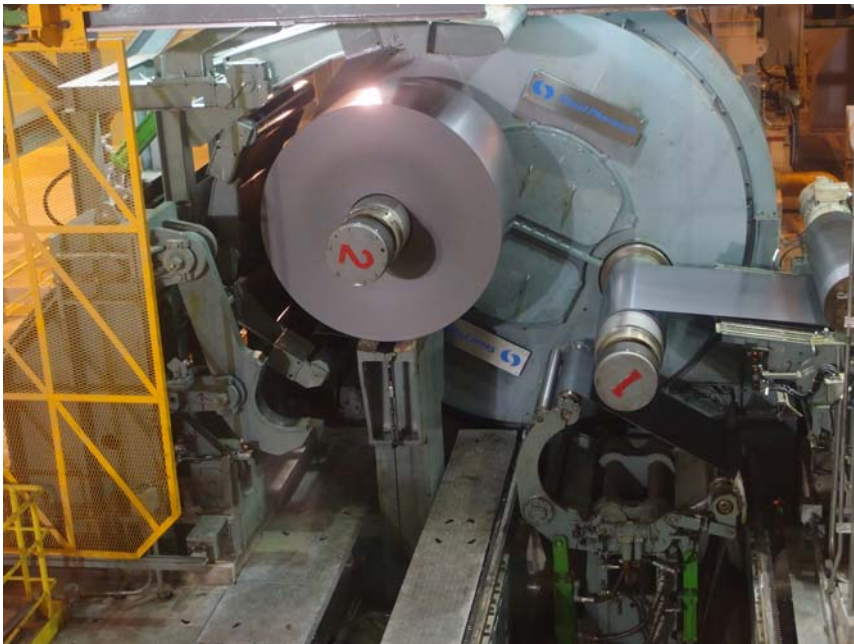
Figure 6 Carrousel Tension Reel
