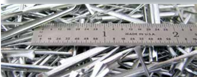
The HV1 1's long length creates lengthy, needle-like chips in aluminum.
