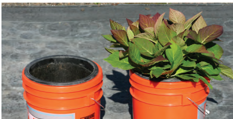
Figure 2. Buckets are used to capture applied irrigation water and leachate. The plant container needs to nest in the opening of the bucket lid. The mating between the container and lid should not allow water to enter the bucket. Putty or caulk may need to be used to exclude the water.
