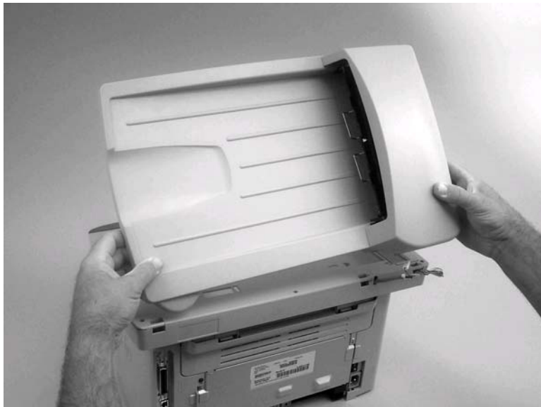
Figure 5-58. Remove the flatbed lid (5 of 5)
