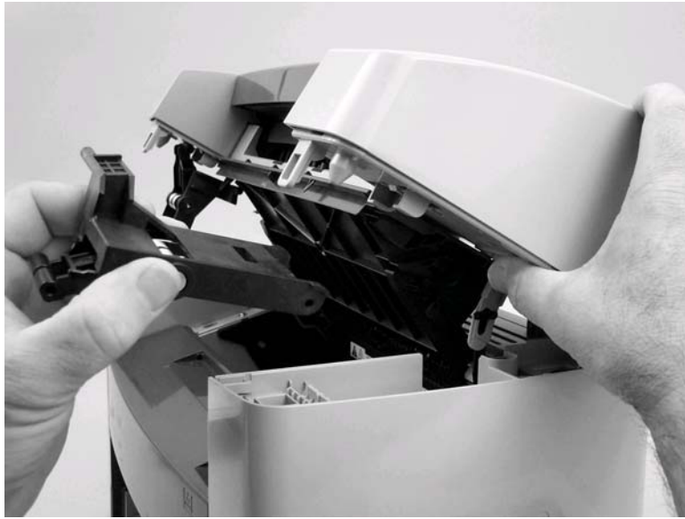
Figure 5-8. Remove the link assemblies and scanner support frame springs (3 of 4)
