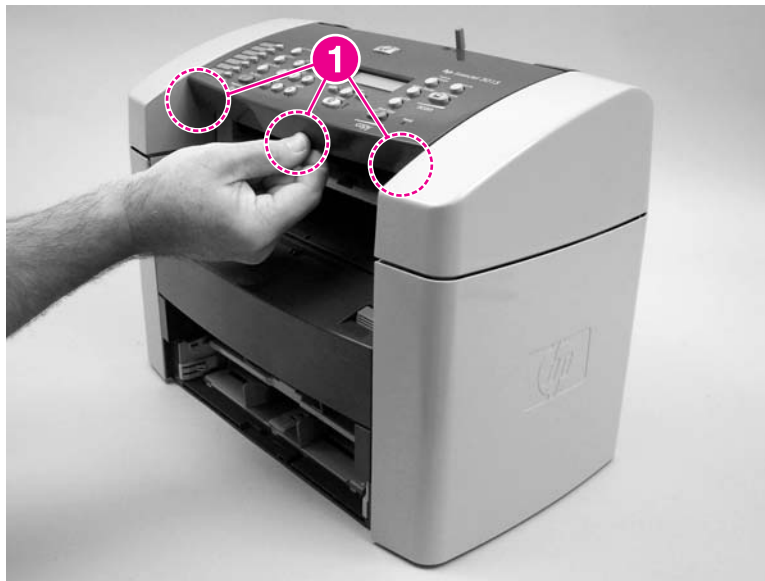
Figure 5-14. Remove the control-panel bezel (1 of 3)
