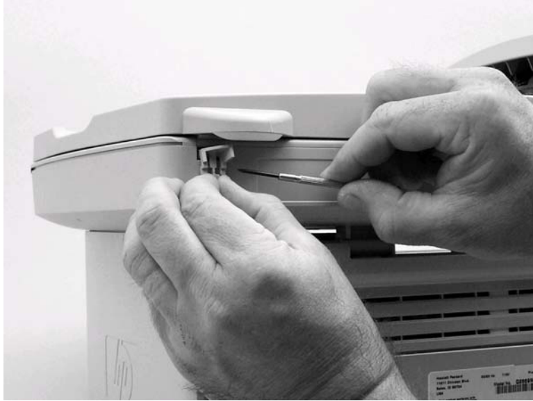
Figure 5-57. Remove the flatbed lid (4 of 5)
