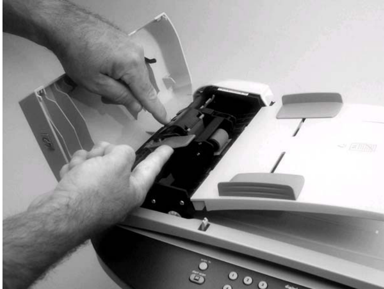
Figure 5-69. Remove the ADF pickup roller (1 of 2)
