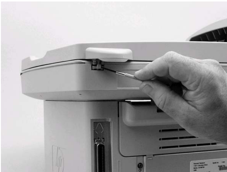
Figure 5-56. Remove the flatbed lid (3 of 5)
