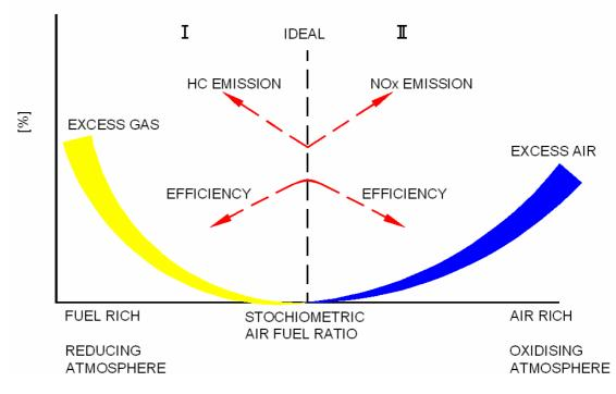
The table above shows the efficiency vs the amount of air / gas introduced to the combustion process. The black dotted line indicates the stochiometric air fuel ratio (the exact amount of air required for the combustion of 1m3 of gas under normal conditions), and is the most efficient way to combust your product and have lowest possible NOx or HC emission.
