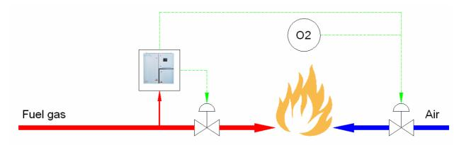
In case large fluctuations in the fuel gas are expected. The wobbe index of the gas flow can be stabilized using the fast responding Wobbe Index signal.
