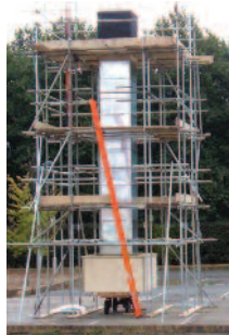
Sunstract system under test in real daylight conditions with integrator box at base
