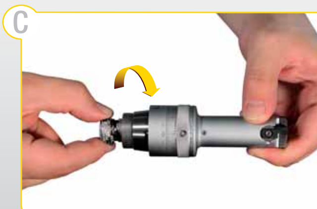
C. Screw the Differential Connector (5) into the rear thread on the Boring Head (1) until the end of the thread. At this time it is not necessary to tighten the Differential Connector (5). Remember that the Differential Connector (5) has two different screws, so there is no way to assemble the wrong side
