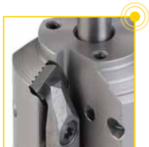
RIQ serration defines valve seat angle
