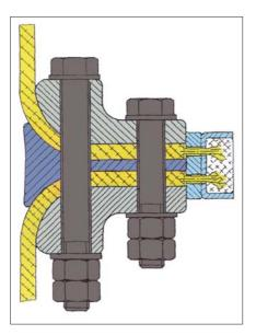
belt clamping connection. As shown on the cross section, the belt is clamped by means of bolts between a steel wedge and two aluminum clamping jaws. The number of bolts depends on the belt width.
