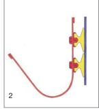
The segments on the back side of the belt are inserted with the belt and the rubber plate into the shaped plate of the bucket back wall, so that the belt is perfectly configured to the diameter of the drive pulley.
