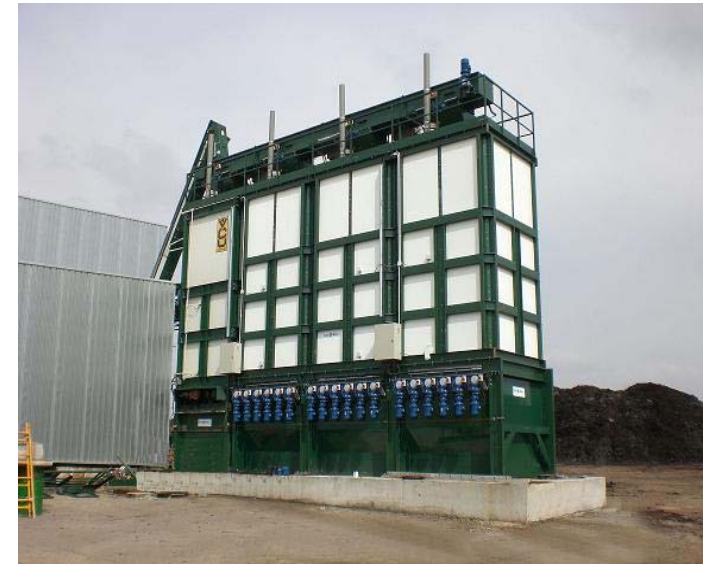
Expanded 4 chamber VCU system
