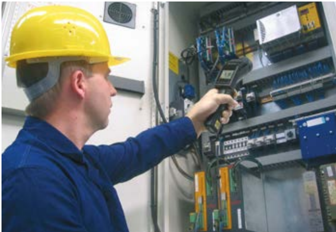
Detailed infrared temperature measurement of an electric control system using the optris® LS integrated close focus optics for 1 mm ranges
