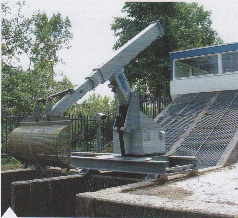
The Bosker Bandit is a mobile solution for smaller pumping stations
