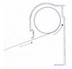
Check that the roof sheet pockets have not folded over – this can cause the fascia not to close on one side.
