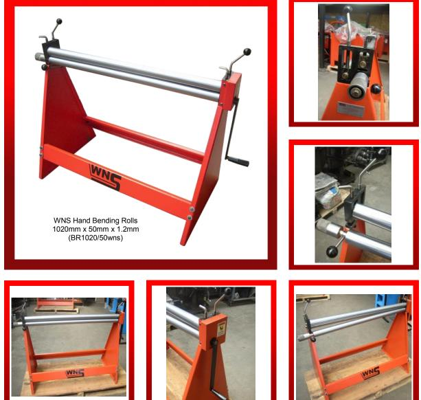
**WNS** INITIAL PINCH HAND BENDING ROLLS (BR1020/50wns) are principally used for rolling tubes/cylinders in sheet metal. The metal is 'pinched' between two rolls and curves as it comes into contact with the third (back) forming roll. The BR1020/50wns has a 1020mm Roll Length, 50mm Roll Diameter and can accommodate Mild Steel up to 1.2mm thick. The rolls are bottom slip, with an Edwards Style fabricated steel frame.
