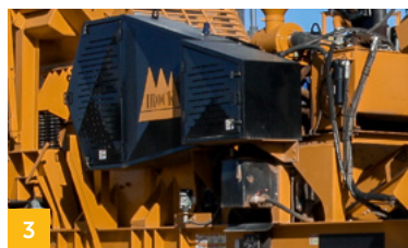
3 A hydraulic adjusting chamber easily adjusts to produce a 2" - 6" product.
