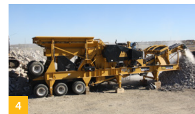
4 Six hydraulic outriggers offer fast and easy off-loading and leveling of the plant to complete setup in less than an hour.
