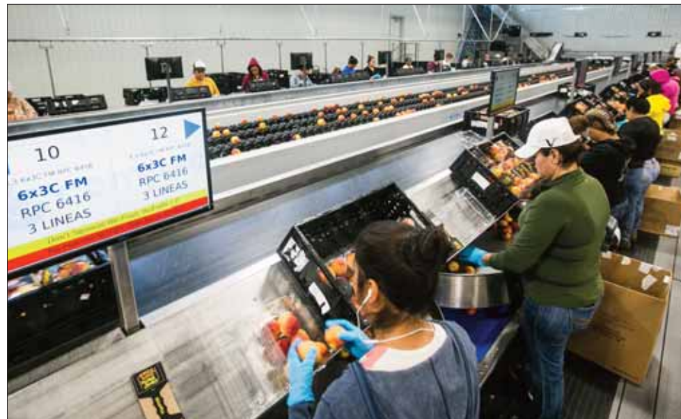
Peach packers can look at a computer screen for the instructions on how to fulfill an order, including packaging and configuration. They also print out the labels for food safety traceability.
