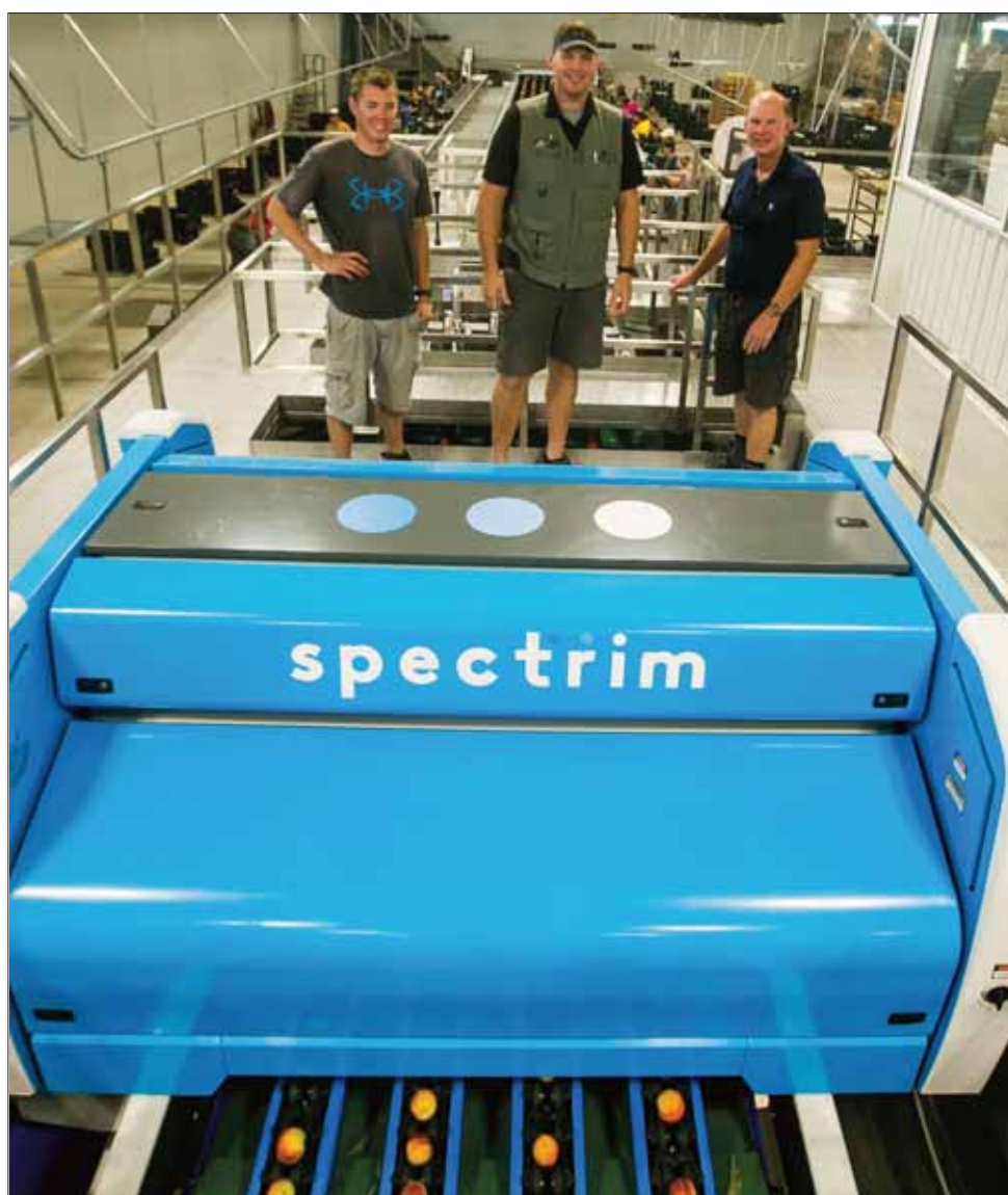
L-R: Jourdan, Ryan and Phil Tregunno stand proudly on their Spectrim vision system which can take up to 500 pictures of each piece of fruit.
