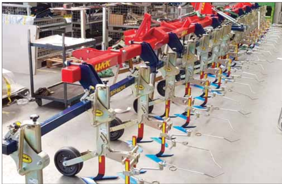
16-row mechanical weed remover for a pumpkin grower. Photo supplied.
