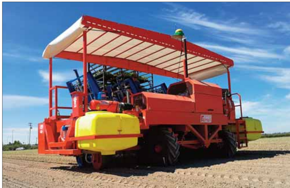
Ferrari Futura fully automated transplanter. Photo supplied.
