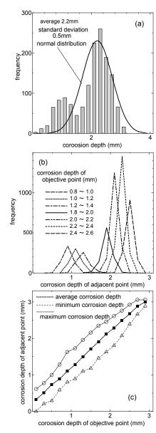
Fig.4. An example of measured results of corrosion depth in the C-bridge
