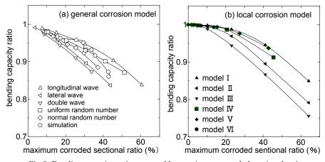
Fig.9. Bending capacity ratio arranged by maximum corroded sectional ratio
