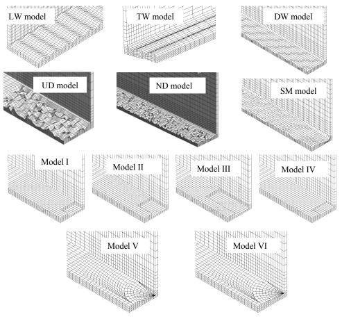
Fig.7. Finite element of each corrosion model
