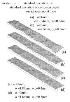
Fig.5. Examples of simulated corrosion surface
