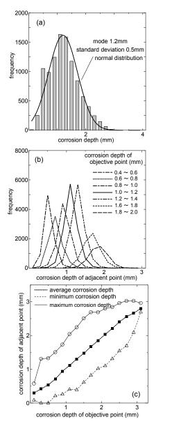
Fig.3. An example of measured results of corrosion depth in the B-bridge
