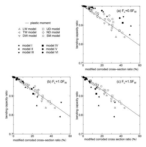
Fig.11. Bending capacity ratio arranged by modified corroded cross-section ratio
