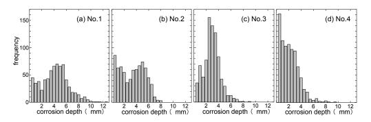
Fig.1. Distribution of corrosion depth on the upper flange of each girder (A-Bridge)
