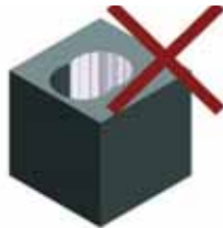
Hole expansion on the centre axis
