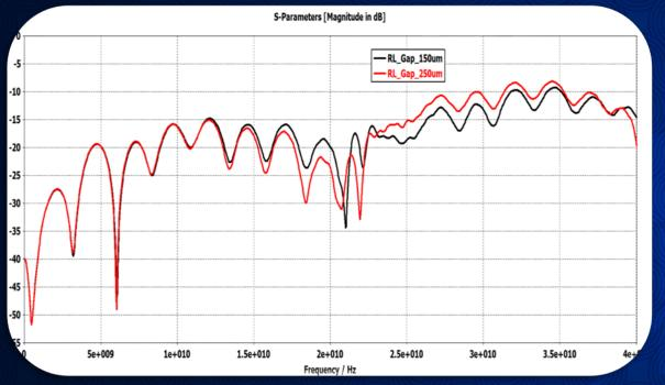
AN1 RL comparison for different air gap between head and wafer
