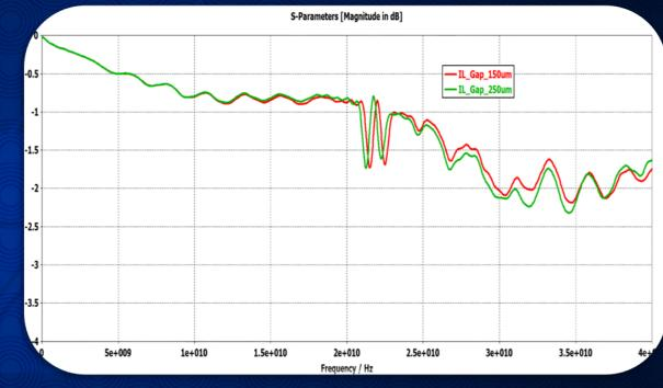
ANT1 IL comparison for different air gaps between head and wafer
