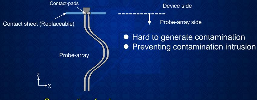
Cross-section of probe-array and contact-sheet
