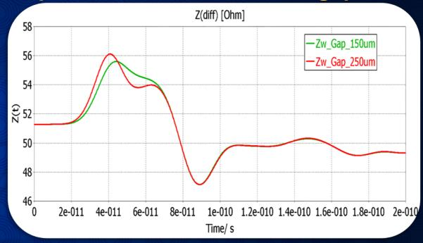
• The air gap between the wafer and the probe head filling material are critical for impedance
