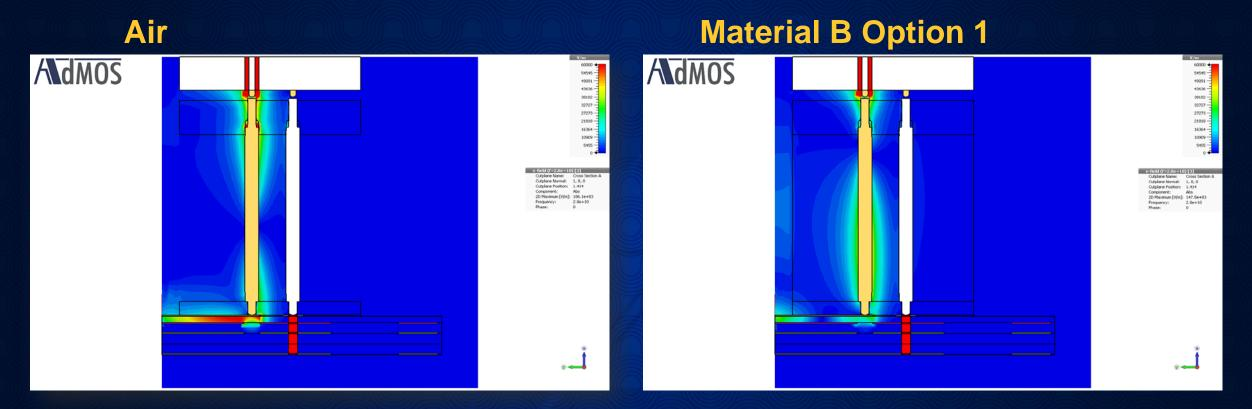
Max EM field intensity with air gap at 28GHz is 186k V/m
