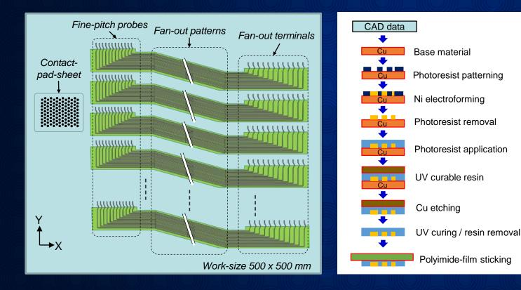
Two-dimensional design and fabrication stage
