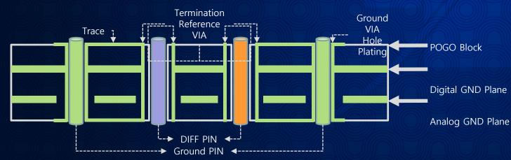
• Using MLB for pogo housing, pseudo coaxial transmission line structure can be attained
