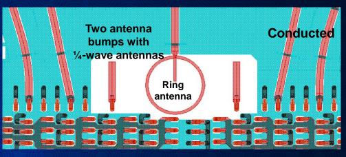
mm Wave Probe Connection: 2 to 1 combining with ¼-wave antennas
