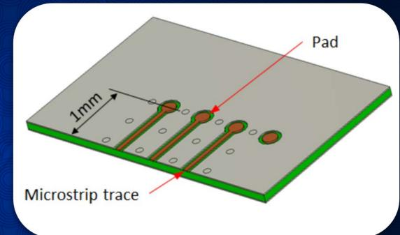
The textbook micro-strip definition of a rectangular conducting cross-section between an inhomogeneous dielectric and air is far away from the reality of an ATE PCB micro-strip geometry
