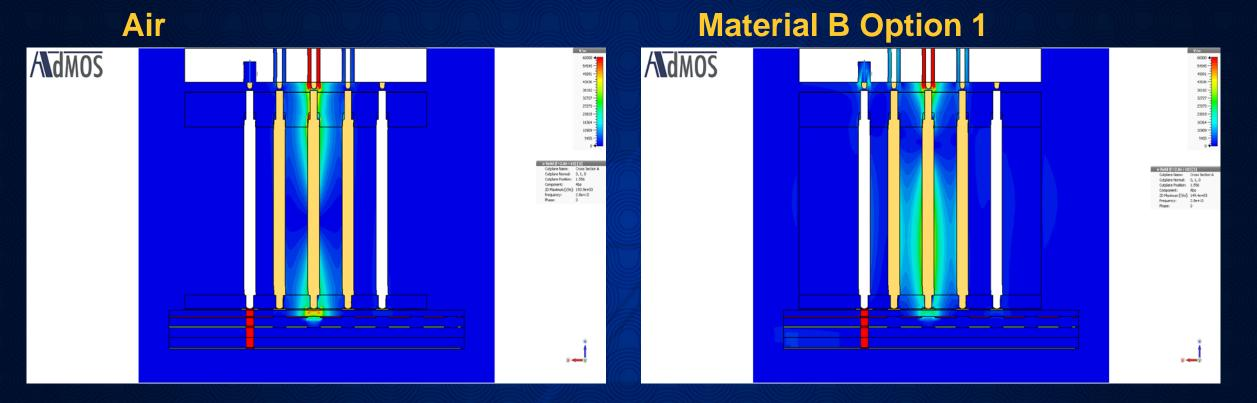
Crosstalk max field intensity with air gap at 28GHz is 193k V/m
