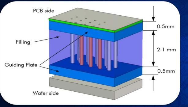
An initial probe head design with air as a filling between guiding plates
