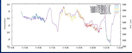
Temperature Changed 2 degree C in 7 days Contact Z Position Changed 60um
