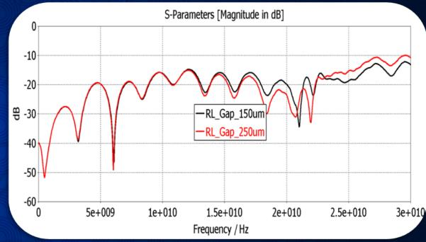
Reduced air gap between probe head and wafer (probe extension) improves IL and RL at high frequency
