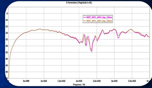
AN1 & AN4 crosstalk comparison for different air gaps between head and wafer
