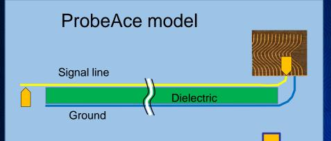
Non-discontinuous micro-strip-line model from probe to terminal
