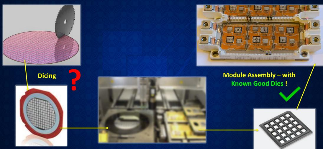
**KGD Test** - Singulated Chips
