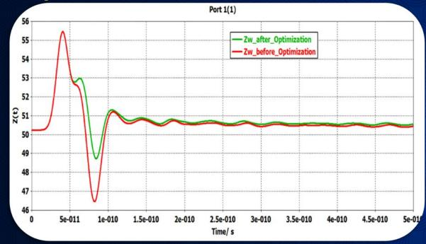
Because of the air gap between the wafer and the probe head body, a non-symmetrical guiding plate construction provides performance improvements as shown in this example
