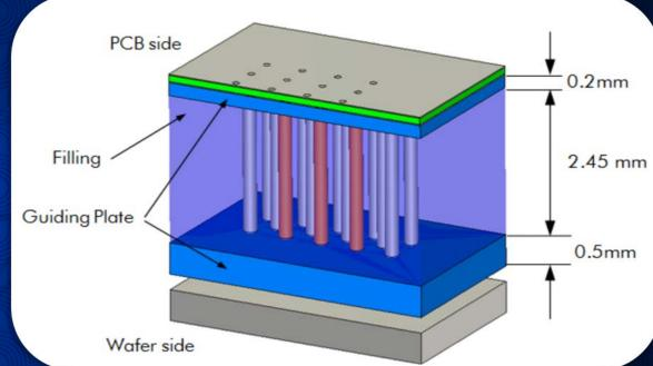
The optimized design with different filling materials and asymmetrical guiding plates
