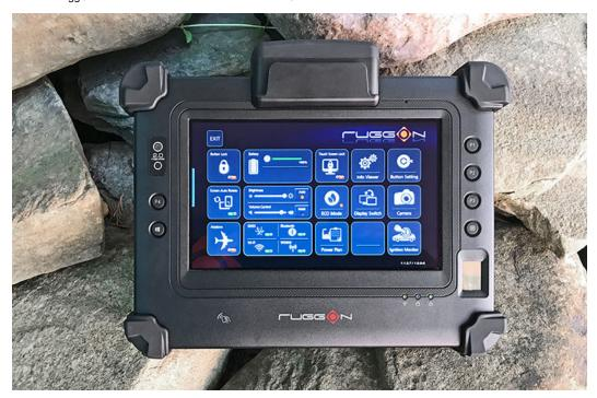
With regard to protection from the elements, the PM-311B carries IP65 sealing where the "6" means it's totally dustproof, and the "5" that it is also sealed against, according to the IP classification system chart, low pressure water jets from all directions. That's far better sealing than standard consumer tablets have.
