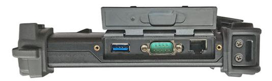
The left side of the PM-311B tablet, shown above, features a full-size USB 3.0 port, a legacy DB9 RS232 serial port, and an RJ45 LAN jack.
