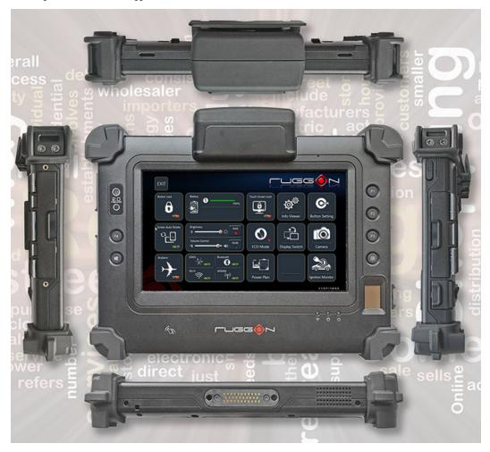
Another indicator that the PM-311B is a seriously rugged device is the protection afforded to all of its ports. It consists of thick hinged polymer plastic doors with rubber pressure seals both on the door side and inside the port openings. Around each door is a double-lipped friction seals. Firmly push the doors inside the port opening until they click into place.
