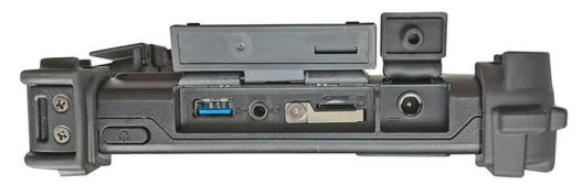
The right side, shown above, has the power button, then an I/O block with a second USB 3.0, a 3.5mm audio in/out jack, a micro SD card slot, and beneath it a micro SIM card slot with a protective metal cover. To the right of that is the power jack with a separate protective cover.
