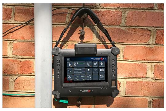
Designed as a very versatile data collection and authorization tool, the PM-311B has onboard WiFi, Bluetooth, GPS, NFC and 4G LTE mobile broadband. It can optionally be equipped with a high-precision fingerprint reader. Depending on its intended application, the tablet can be equipped with optional bolt-on modules. Currently available are two modules, one that combines a 1D/2D barcode reader and a magnetic card reader, one one that combines the magnetic card reader and a MRZ reader.
