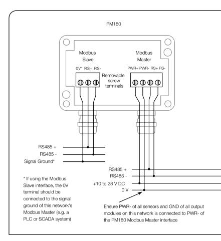
The PM180 has removable screw terminal blocks for the Modbus Slave and Modbus Master interfaces.
