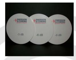
The kit consists of 4 calibrated attenuators, respectively of 3, 6, 9 and 12dB. The purpose is to check the quality of the system by holding an attenuator in front of the receiver box. In this position, the attenuator will degrade the signal coming from the parabolic reflector.
