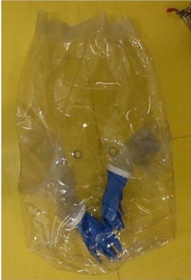
There are spray nozzles at the front and the back of the glove-change-bag to enable easy spraying of sleeve and clamps
