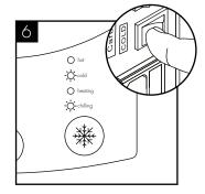
When the cold water switch is turned on, the cold water and chilling LED will be on.
