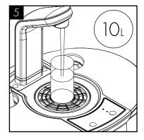
Flush through approximately 10 litres of water. Check and adjust the CO2 pressure accordingly.
