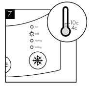
The temperature of cold water can be set from 4c to 10c. When the chilling LED is off the set temperature has been reached. This can take up to one hour.
