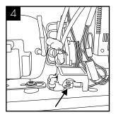
Locate the Leak Detector valve.
