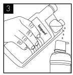
Add 25 ml of Bioguard Internal Sanitisation fluid to a clean and empty service filter cartridge.
