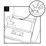
Locate the detection probe which can be found in the bottom at the rear of the machine. Dry the probes and internal area with a dry cloth.
