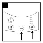
Briefly press cold/ambient dispense button to release internal water pressure from the machine.
