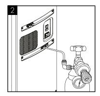
Connect the assembled CO2 bottle and regulator to the machine using 1/4 inch pipe.
