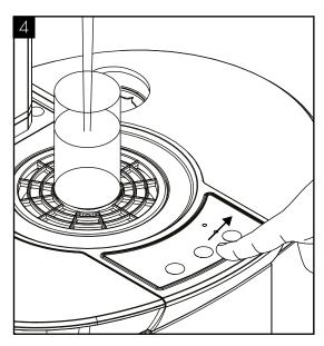
Ensure to release the Sparkling water button and take care to avoid releasing excess amounts of  ${\it CO2}$  gas.
