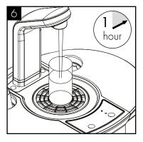
It will be necessary to leave the machine for up to 1 hour for sparkling water to develop, by absorbing the CO2.
