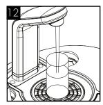
Pre-flush the new filter to waste using the ambient button (and sparkling button if present) until the water appears clear and is free of air. Flush through a small amount of water to check all functions.
