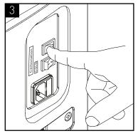
After completing the water installation, turn on the soda power switch and the pump will run. Do not open the regulator valve until the carbonated switch has been turned on.
