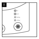
When the heating LED is off the pre-set temperature has been reached. This can take up to 30mins.
