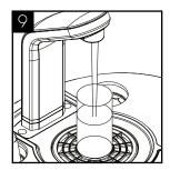
When the external cleaning (minimum 5 minutes) is completed, flush the machine using the cold button with clean water until the dispense water runs clear. Repeat briefly with the ambient button (and sparkling button if present).
