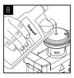
Remember to include the drip tray. Empty the Waste Overflow System and flush through with a small amount of sanitisation fluid if needed.
