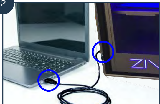
Connect USB or Network Cable
