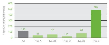
**Fig. 3**—Resistivity improvement differs between types of ion exchange media. EPT's proprietary ICB ion exchange media (Type E) provided the best average resistivity improvement.
