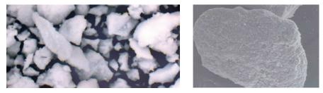
**Fig. 1**—Selexsorb GT alumina-based adsorbent (ABA) under 4x (left) and 120x (right) scanning electron microscopy (SEM) magnification showing abrasive aluminosilicate particles.
