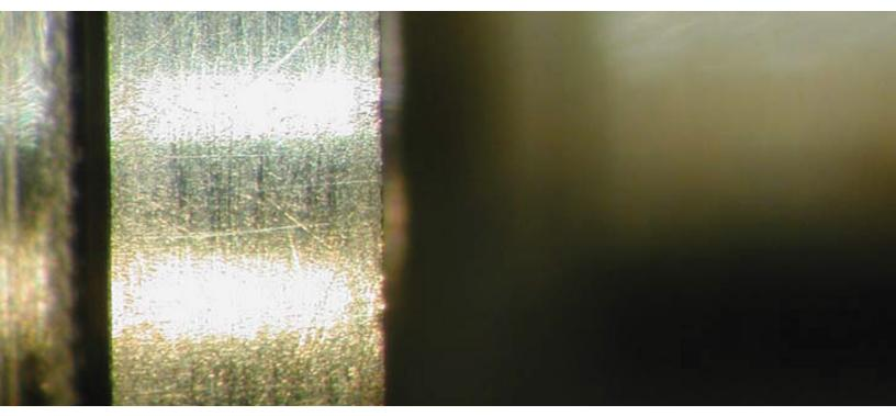
Photo of the spool null edge showing damage consistent with electron stream erosion.
