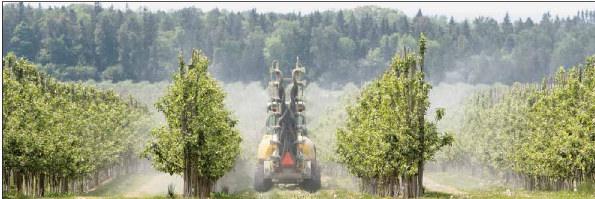
This HOL sprayer, designed for high-density apple orchards, is pictured at petal fall at Scarlett Acres, Colborne, Ontario.
