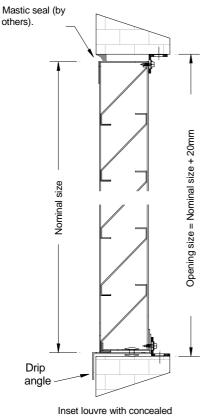
Inset louvre with concealed (internal) fixings for high security application.
