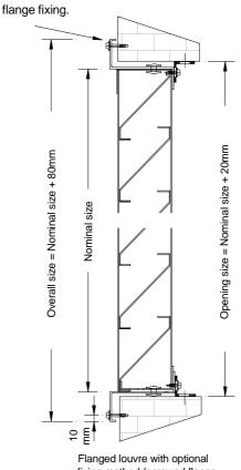
fixing method (screwed flange or concealed).
