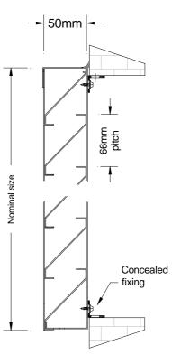
Surface mounted louvre with concealed (internal) fixings for high security application.
