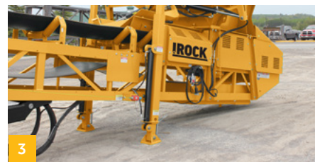
3 Hydraulic Axle Jacks enhance stability while the stacker is in operation. Hydraulic Axle Extensions attach to the rear undercarriage and enable axle extensions/contractions.
