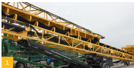
1 Straightforward hydraulic controls to fold and unfold, raise and lower the conveyor.
