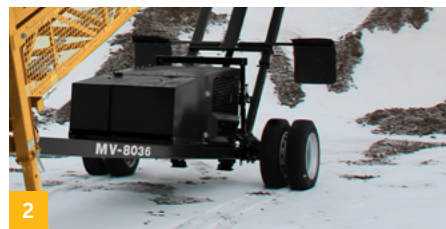
2 Pivoting axle box allows for creating swept radius stockpiles.
