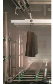
Water which has adhered to the product (material) during transfer is dried off.
