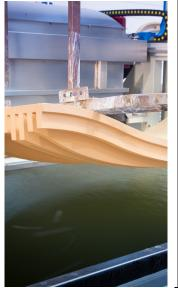
Having fulfilled its role as the medium for the print transfer, the film is washed away.
