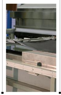
The film is specially treated to activate the inks. The film is activated by an autonized Patented Activator, release by high pressure guns.
