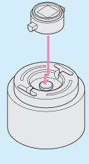
To prevent components with a correct orientation from being turned in the  $\theta$  direction when being inserted.
