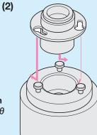
To install components with a correct orientation rotated to a specific angle at a constant moment' after insertion.
