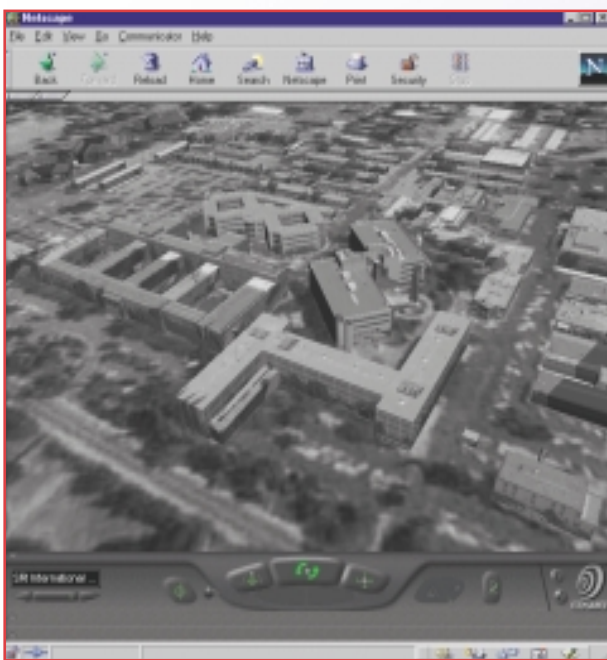
A texture-mapped site model of the SRI International campus that has been georeferenced onto an underlying terrain model. Note the accurate alignment of the latitude/longitude-specified buildings with the underlying 1 m resolution USGS DOQ satellite imagery in UTM coordinates.
