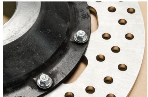
... > Flat washer > Nut. Torque tighten the nut to 6 Nm.
