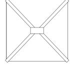
Maximum size Contemporary Pyramid lantern as per line drawing above =2000mm x 2000mm. The Regular Pyramid lantern can go up to larger sizes with additional rafters.
