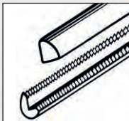
Infant CV with unique half-moon shaped jaw profile for increased clamping stability (no twisting of jaws)
