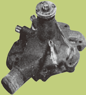
Fig. 1. Evidence of seal leakage from weep hole.
