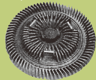
Fig. 6. A worn fan clutch rob power by remaining fully engaged.
