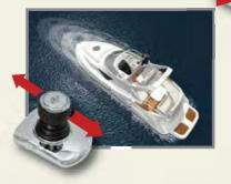
Move the Axius joystick toward the bow or stern of the boat to move directly forward or backward.
