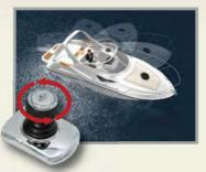
Twist the Axius joystick to turn the boat within its own length. An ideal maneuver for changing directions in a tight space.
